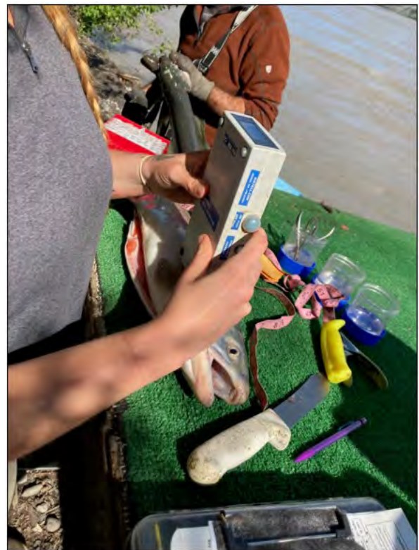
Figure 4. ADF&G fisheries technician using a “fish fat meter” to non-destructively measure fat content of a sockeye salmon harvested in the Glennallen Subdistrict subsistence fishery, 7/7/2023.
