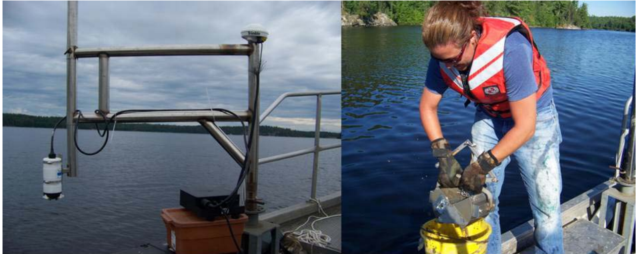
Figure 4. a) Acoustic Doppler Profiler (ADP) equipment used to map velocity profiles in areas of interest. b) SDSU graduate student Stephanie Shaw taking a substrate grab.
