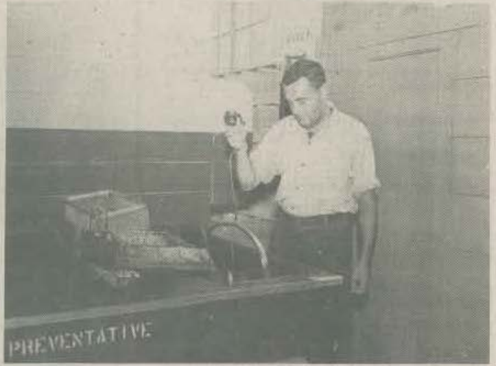
Rust preventive is applied by dipping in teryle grade 2 or grease grade 'A', as being done by Jack Kawasky, SKT3/c.
