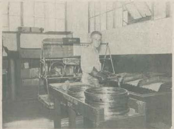
Cleaning material with Stoddard Solvent against all foreign matter being performed by Frank L. Dorran, S2c.
