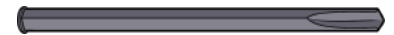
rock drill: used to create a hole that would be filled with explosive powder; once ignited, this powder would blow up rock to make way for construction; one or two men would drive this drill into rock with a sledgehammer
