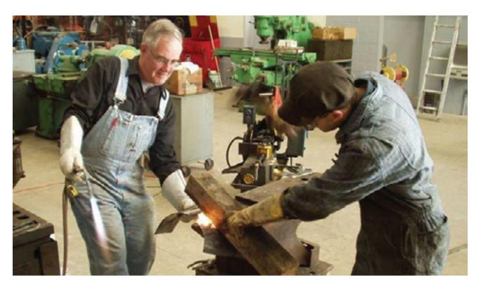
Two B&O Railroad Museum Restoration Shop craftsmen fabricate a piece of the smokestack for the B&O #305 Davis Camel locomotive, one of two surviving "camel" type engines in the world. The restoration of this locomotive, as well as the seven other extremely important steam engines, was needed after the B&O Railroad Museum's roundhouse roof collapse in 2003. Partial funding for the restoration came from the City of Baltimore through the BHAA Small Capital Grant Fund.
