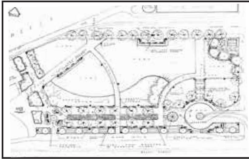
east side of the park and on the north side of the cable car landing, connecting the north side of the park with the water and Hyde Street Pier. Included in the drawing set were details for the cast iron benches, gas-lamp streetlight fixtures, raised planter boxes, metal tree grates and guards, and wrought iron hand railings. The paths and plaza were paved with crushed gravel.<sup>59</sup>
