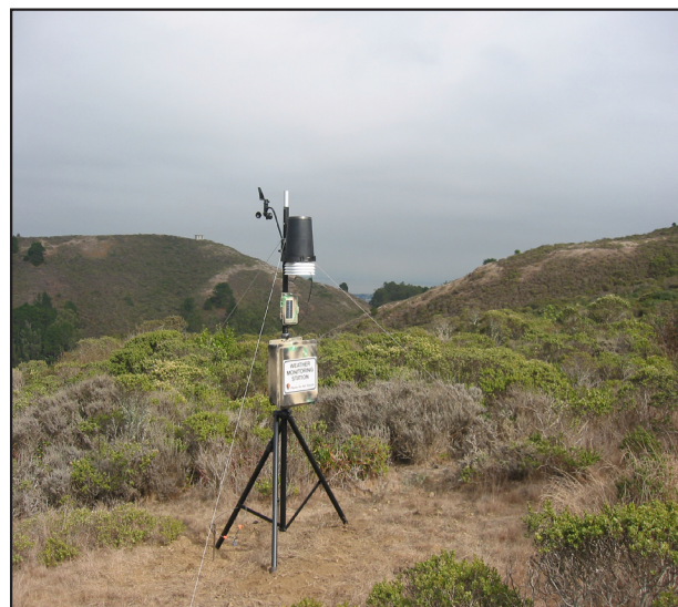
Weather monitoring stations take many different forms and measure parameters such as temperature, precipitation, humidity, and wind speed.
