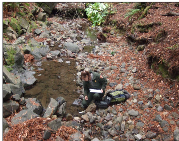
SFAN staff samples water for temperature, dissolved oxygen, pH, specific conductance, discharge, coliform bacteria, and nutrients.
