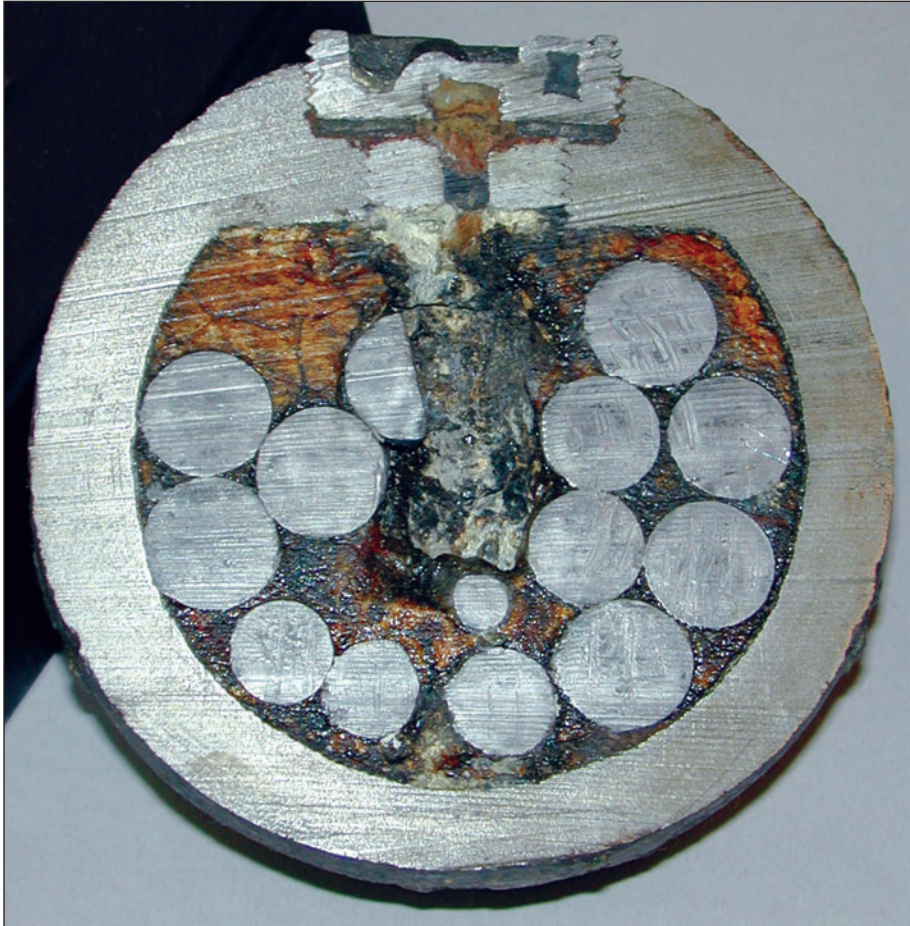
Figure 6. Cut away of Bertrand 12-pounder case.
