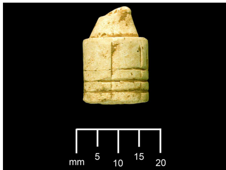
Figure 13. A .58-caliber Minie ball with extreme ramrod marks and heavily engraved rifling marks from a M1855 rifled musket (FS2789).
