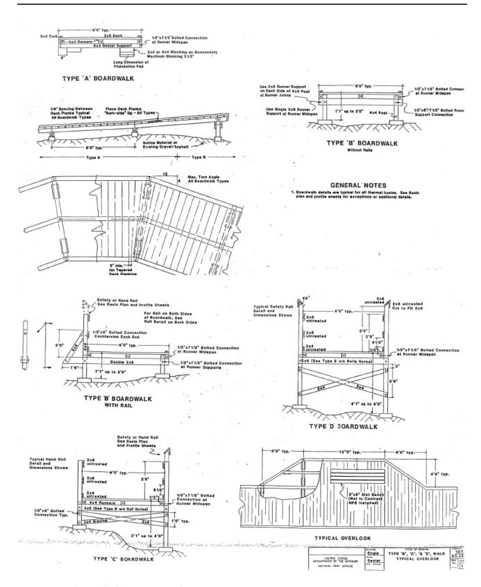
Figure 4.11: Specifications for floating boardwalk for trail around pond.
