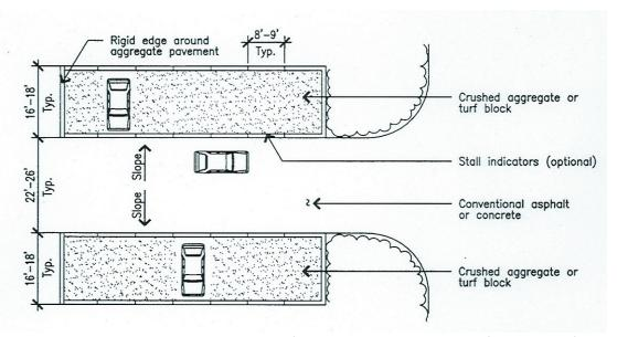
Figure 4.4: Hybrid parking lot example. Parking surface may be crushed aggregate or turf block instead of an impervious surface like asphalt.
