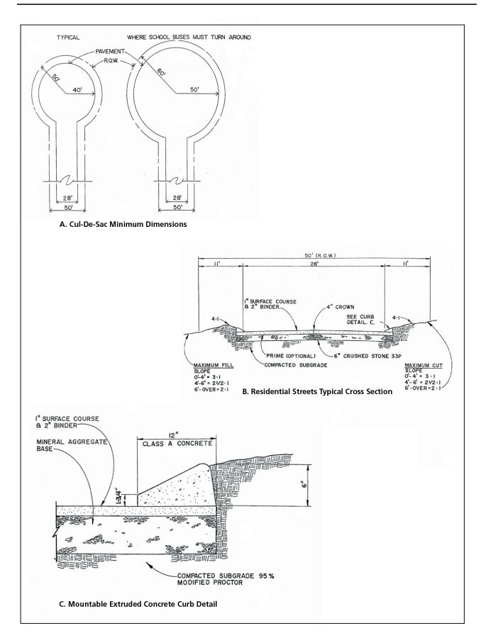
Figure 4.2: Typical cul-de-sac specifications. Mountable curbing facilitates turning, backing up, and parking of larger vehicles.
