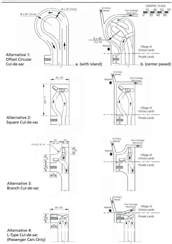
Figure 4.1: Alternative parking lot designs for Victory Woods (OCLP, 2006). Alt. 1-4 include 2 disabled parking stalls, and Alt. 1-3 faciltiate drop-off and turning/backing up of a small bus up to 30' in length. With Alt. 1, the area can be reduced if the center is paved.
