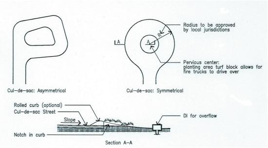
Figure 4.3: Typical cul-de-sac specifications. Asymmetrical cul-de-sacs are often used for suburban or rural settings.
