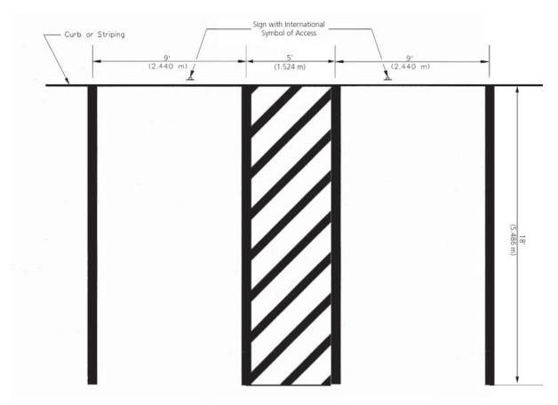
Figure 4.5: Specifications for two disabled parking stalls.
