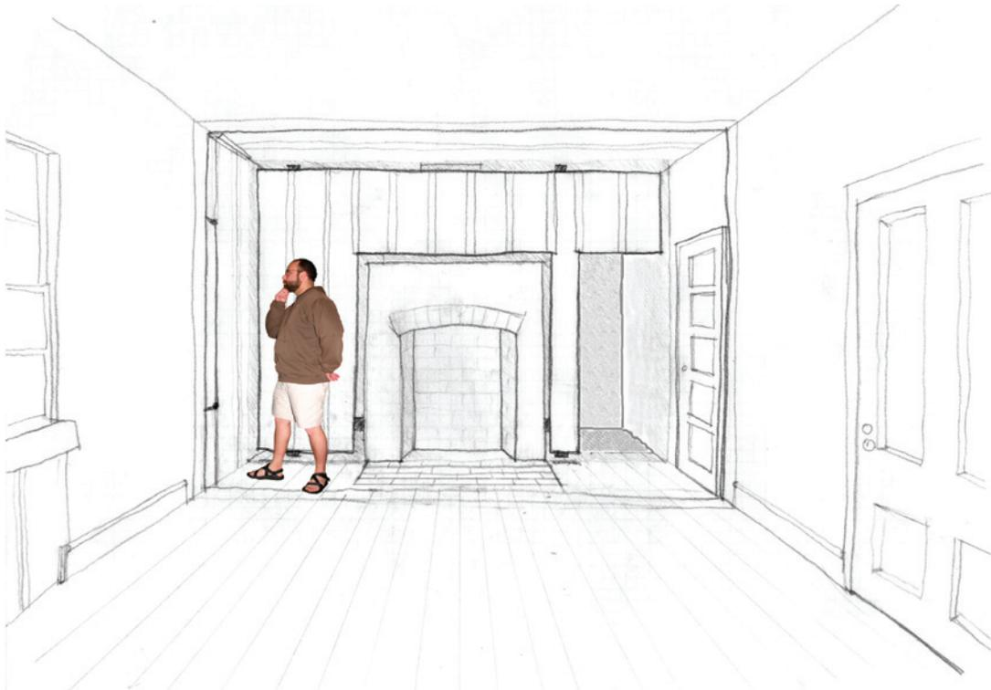
Fig. VII-3. Perspective drawing showing the interior of the proposed spatially-restored Room 1 looking south. Looking through the doorway to the right of the hearth, the intrusion of the walls from the twentieth century restroom can be seen. Beaver Board is depicted as partially removed in the current Room 2 (E5).
