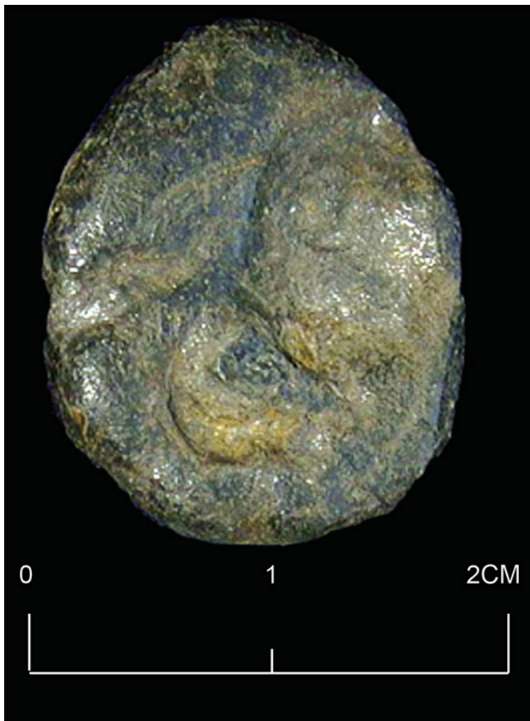
Figure B3. The head of the .58-caliber bullet showing the impact deformations and scars.
