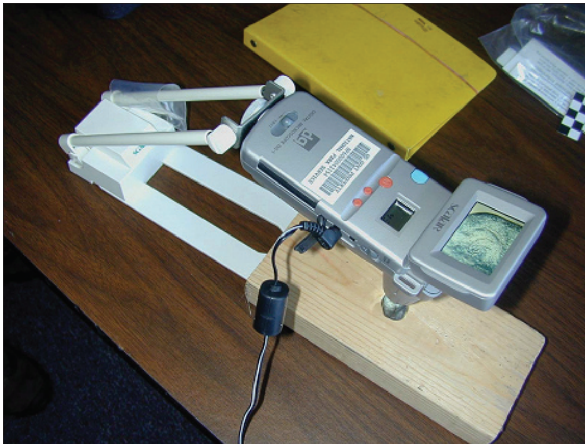
Figure B5. The portable digital microscope in use at Pea Ridge National Military Park with the McCulloch bullet displayed on the screen. The magnified image is captured and stored on a Compact Flash media card in standard jpeg image format.
