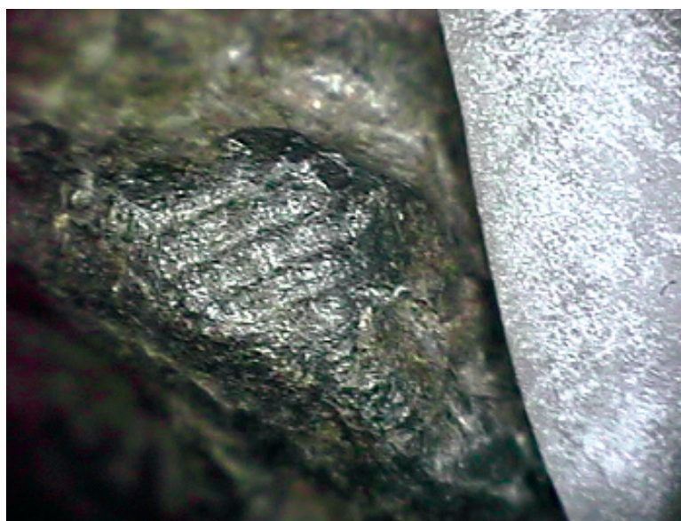
Figure B6. The very fine toolmarks on the side of the impact deformed head. The marks are consistent with the gripping surface of Civil War era medical forceps.
