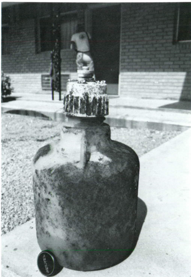
Fig. 10. Another microbiological sampling unit in which nearly all the water was expelled by gas production.
