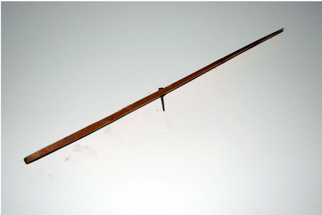
Figure 1.3A-2. Portion of original wood shingle and machine-cut nail, as found in Attic 301.
