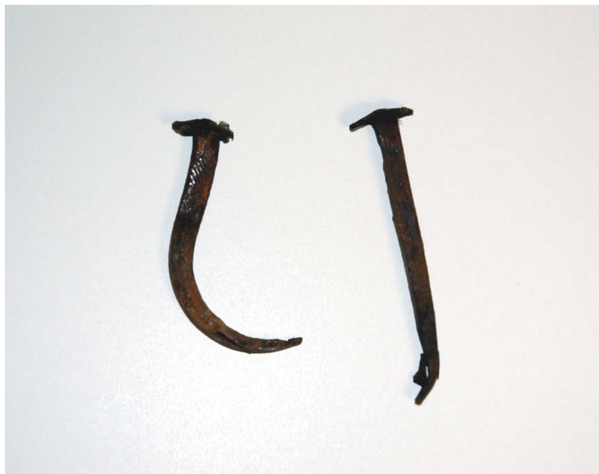
Figure 1.3A-41. Hand-wrought nails found in the horizontal board wall.
