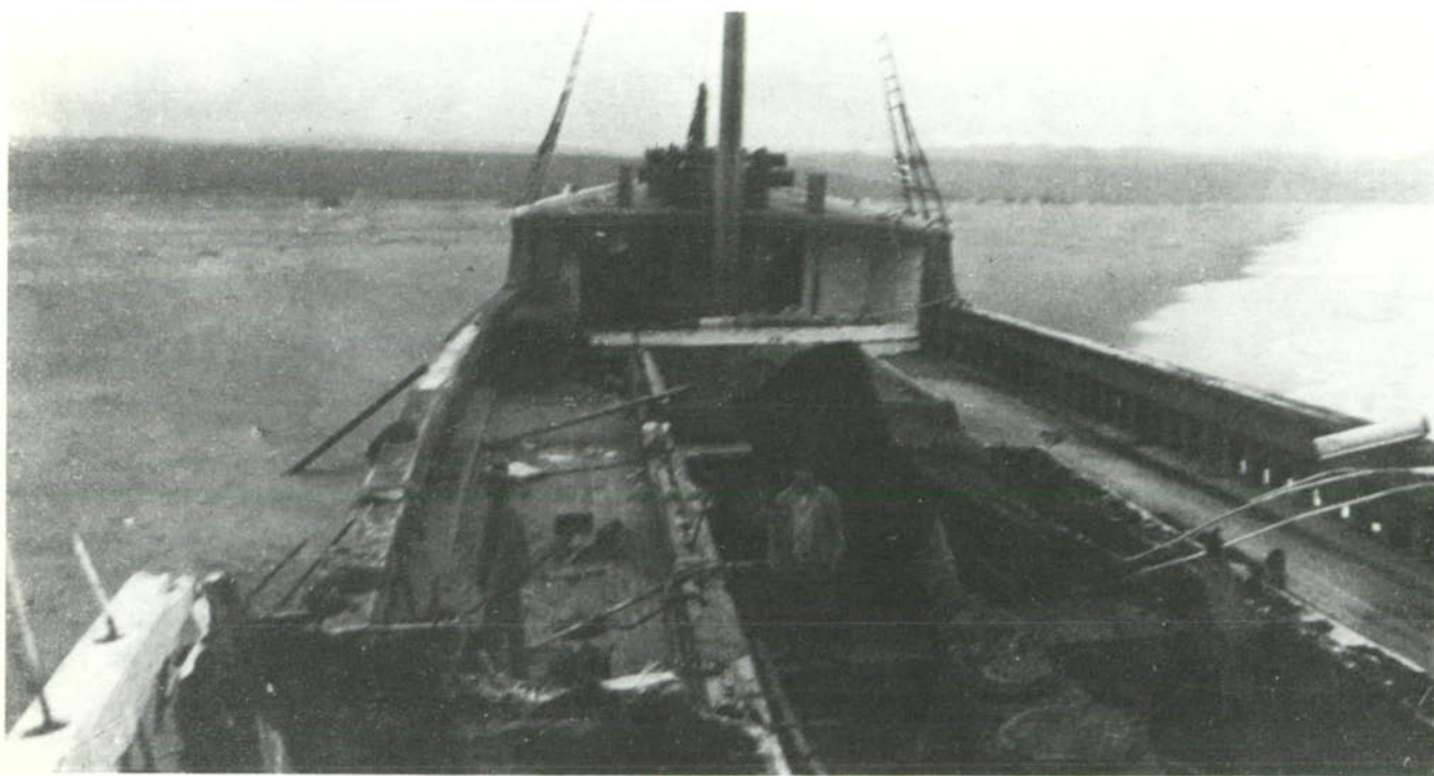
Plate 6. Deck view looking forward on S.S. Pomo . Pomo 's engine can be seen in the foreground. The boiler can also be seen. The forecastle deck and a small portion of the starboard hull, shown in the photograph, were observed on the beach in 1983 (Appendix II). Photograph by Clara Marshall, National Maritime Museum, San Francisco.
