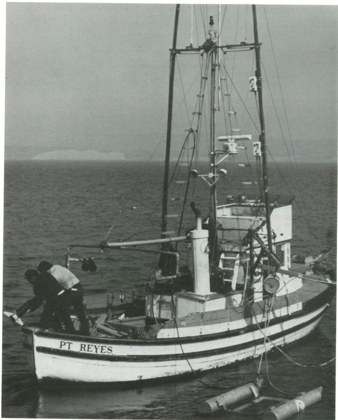
Plate 29. Local fishing vessel Nick used as the survey vessel during the second field session. The magnetometer sensor is being deployed. The pontoons off the starboard support the sub-bottom profiler sensor and the side scan sonar towfish can be seen on the stern.
