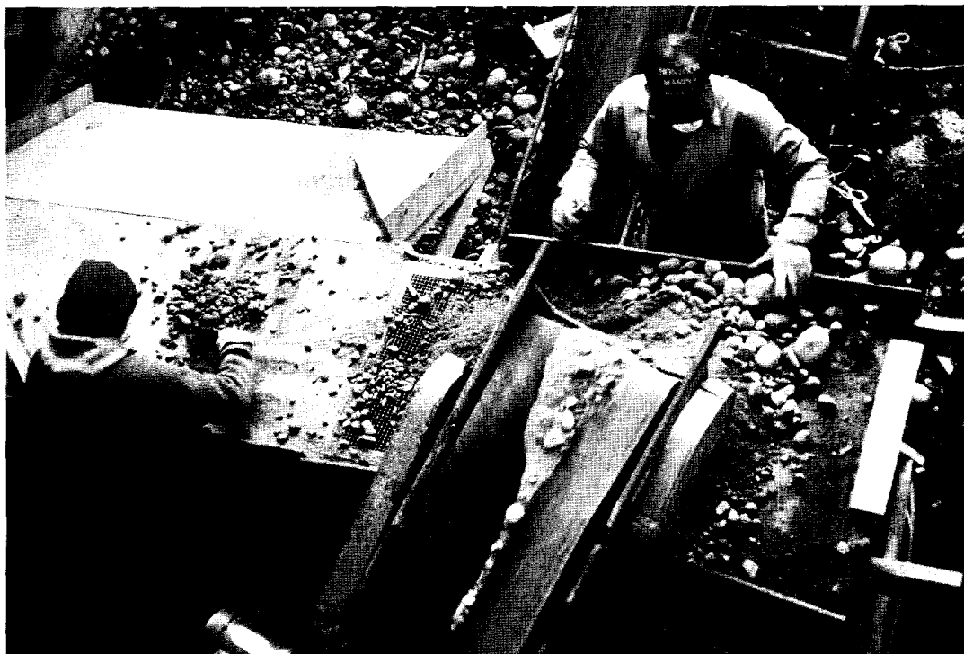
Figure 53. Photograph of conveyor belt and screen table assembly. Note the large mesh of the screen.
