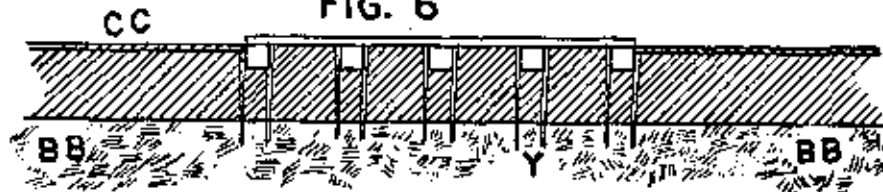
PLATFORM LAID ON FILL
