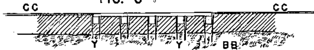
PLATFORM PLACED ON FILL
