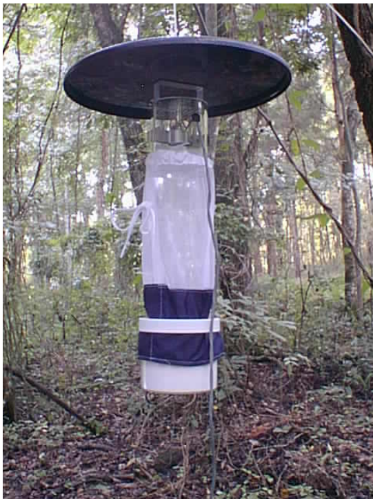
Figure 3. CDC Light trap with collection container.
