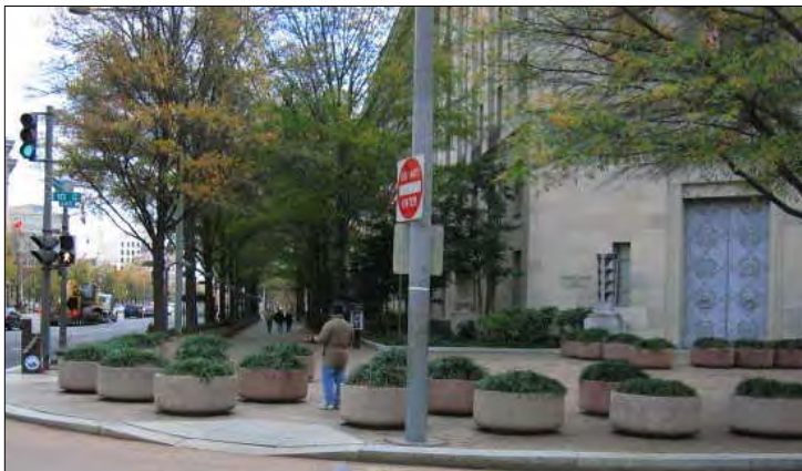
Planters are used as security barriers.
