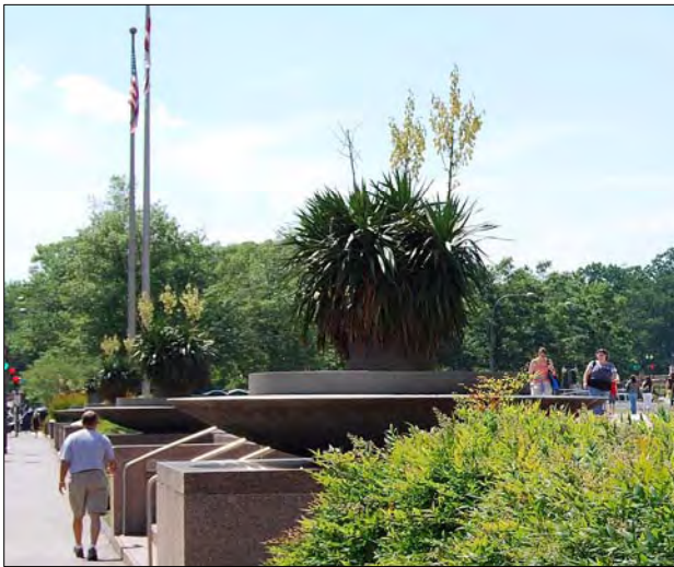
A variety of concrete planters are used along Pennsylvania Avenue, both as decorative highlights and as security barriers.
