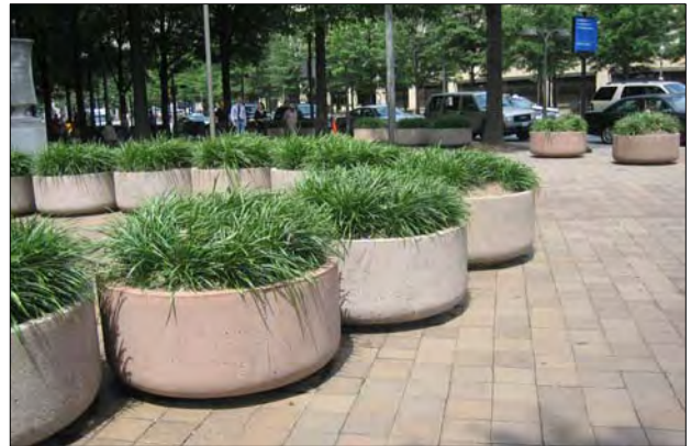
A variety of concrete planters are used along Pennsylvania Avenue, both as decorative highlights and as security barriers.
