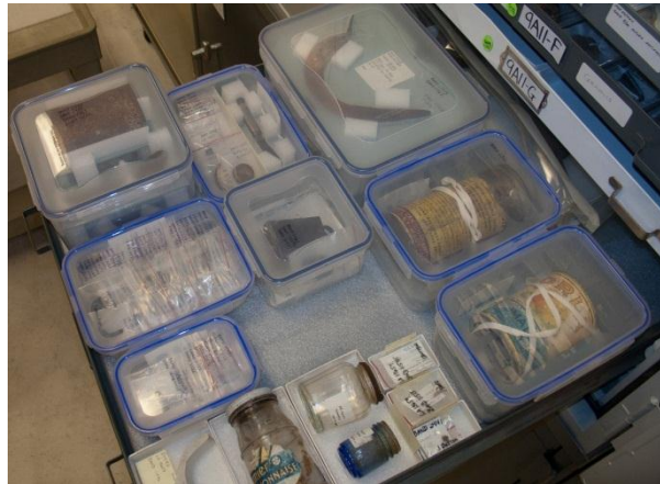
Figure 7.11. Specialized Microclimate Storage. Objects housed in plastic containers in a cabinet drawer. Containers provide buffering against RH and temperature fluctuations.
