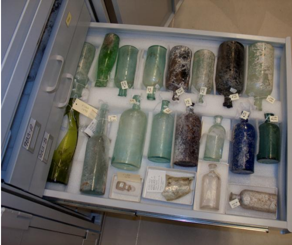
Figure 7.8. Bottle Storage. Bottles anchored in custom made ethafoam at the neck in a cabinet drawer.
