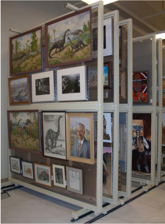
Figure 7.15. Painting Rack Storage. Painting and framed 2-D items rack constructed of slotted angle iron and 2" mesh welded wire fencing.
