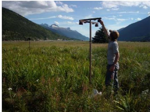
*Passive ambient concentrations sampling for various oxides of nitrogen and sulfur with Ogawa filters.*
