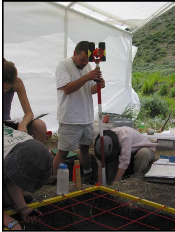
Figure 4. Earthwatch volunteer James Macomson holding prism while artifact is mapped with EDM (3 July 2003).
