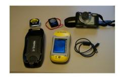
Facilities Management GPS Data Collection With Trimble Geo XT and Geo XM Units
