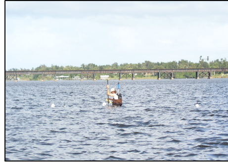
Figure 4. Researcher collecting data points with the RTK GPS rover unit on a reef within the Sebastian River. Note the Florida East Coast Railroad trestle in the background.
