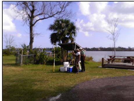
Figure 3. Researchers setting up the RTK GPS base station along the shore of the Sebastian River.
