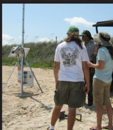
The camera array is a light-weight, mobile platform constructed out of aluminum to hold the camera, battery box, solar panel, and transmitter. The array had to be sturdy enough to withstand exposure to the elements on the beach for months at a time and easy enough to be repositioned from nest to nest by one ranger.
