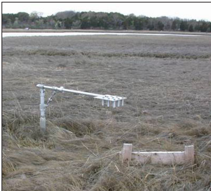
Figure 1. A typical permanent station on the marsh surface at Nauset Marsh with the SET.
