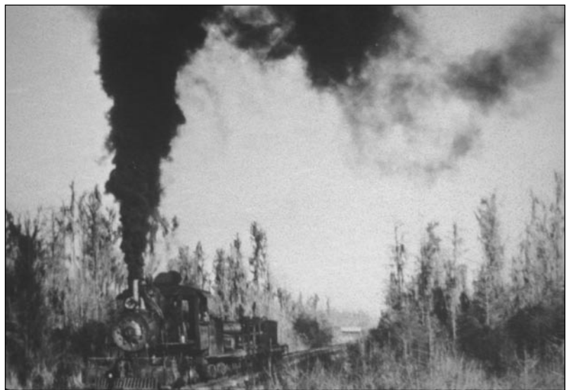
Narrow gauge trains were instrumental in hauling cut timber out of the swamp. Eventually 35+ miles of track were laid. The cut lumber was hauled to the north using rail as well.
