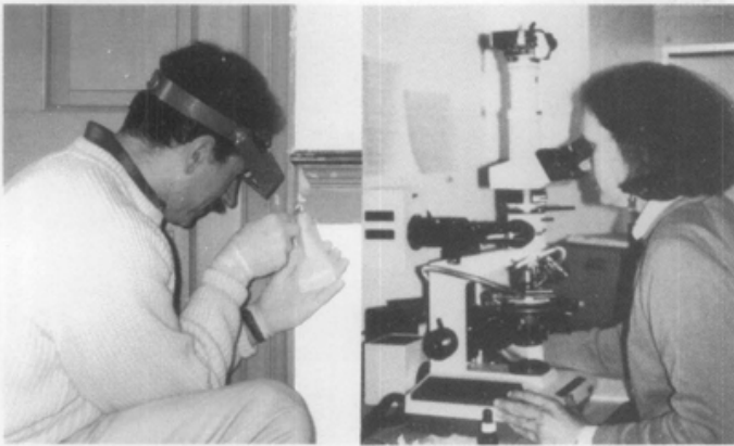
A B Figure 9. Conservators are shown in the two-part process of conducting a complete paint investigation: (a) Paint samples are carefully collected onsite. (b) In the laboratory, an ultra violet light microscope is used to identify pigment and binding media. Paint samples are photographed with the camera mounted on top of the microscope. (right). Photo left: Courtesy, Matthew J. Mosca; Photo right: Courtesy, Andrea M. Gilmore.
