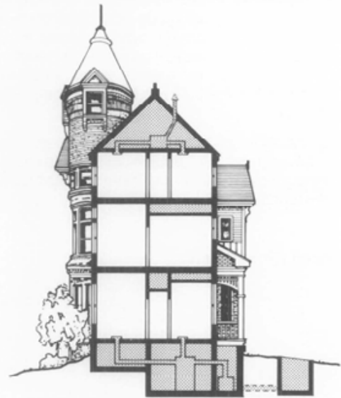
8. In considering options for new systems, existing spaces should be evaluated for their ability to house new equipment. This sketch shows several areas where new mechanical equipment could be located to avoid damaging significant spaces. Sketch: NPS files
