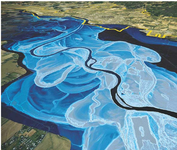
Figure 1.08. LIDAR topography mapping used to document the historic channels of the Willamette River near Corvallis, Oregon (Image by Oregon Department of Geology and Mineral Industries, 2010).
